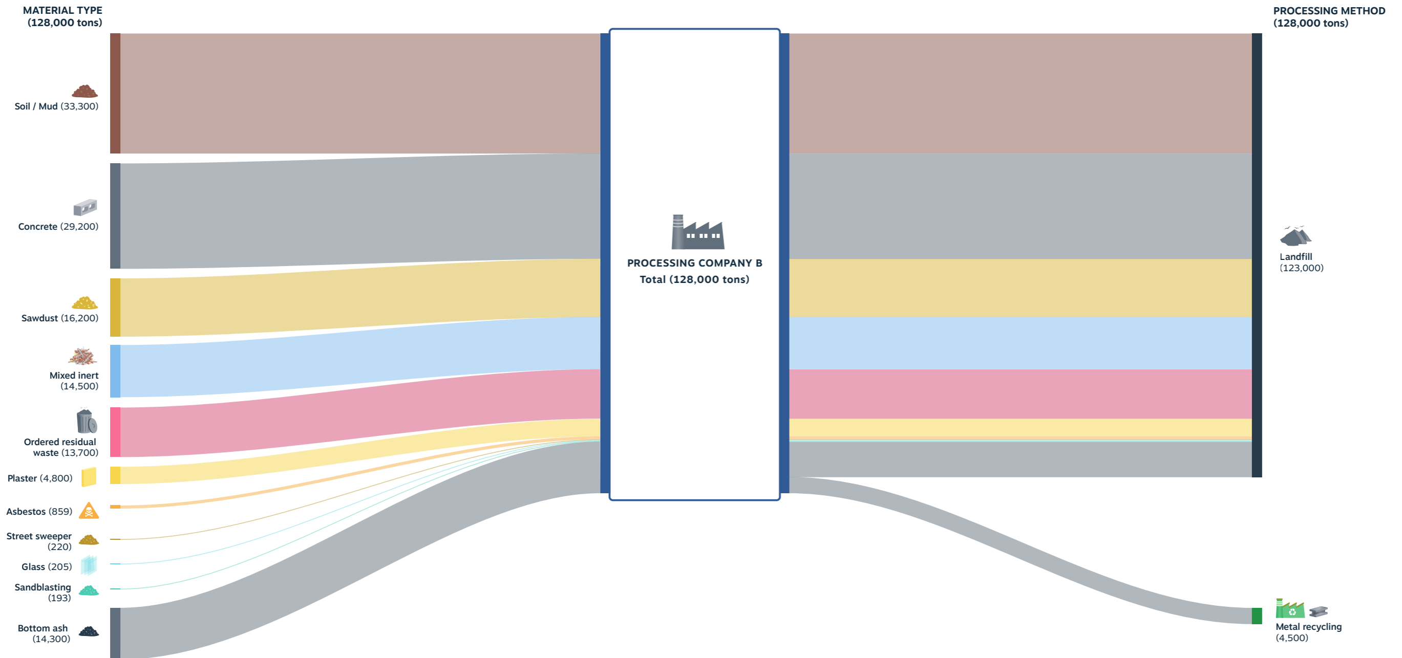
Figure 20 Material flow analysis for the waste processed by Processing company B including on the left side the type of materials received and on the right side the processing method. The colours indicate the type of material, the thickness of the flows are in proportion to their mass. The mass is in tons and the data is for the year 2023.
